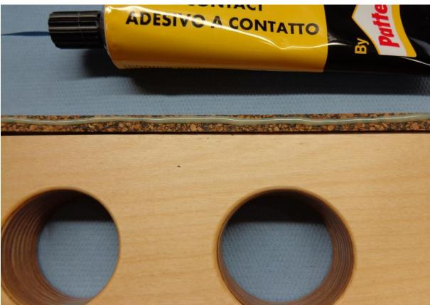
**6.** Apply contact adhesive to the surface of the valve cover
