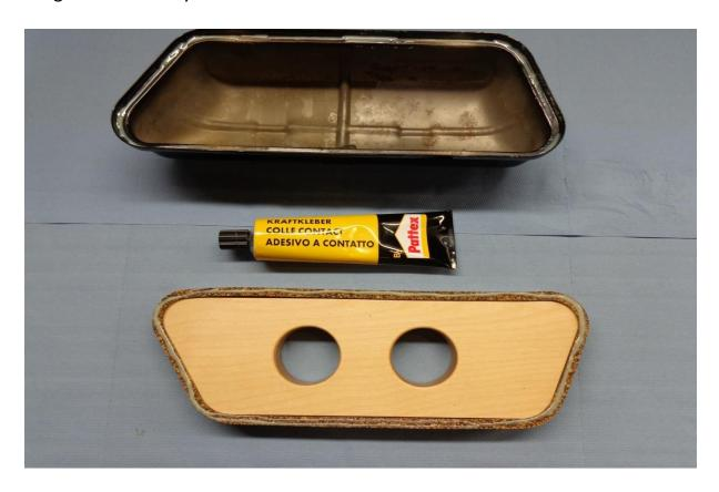
**8.** Place the gasket tool on the valve cover (fits exactly!)
