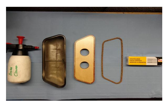
**2.** Degrease the inside of the valve cover with the brake cleaner.
