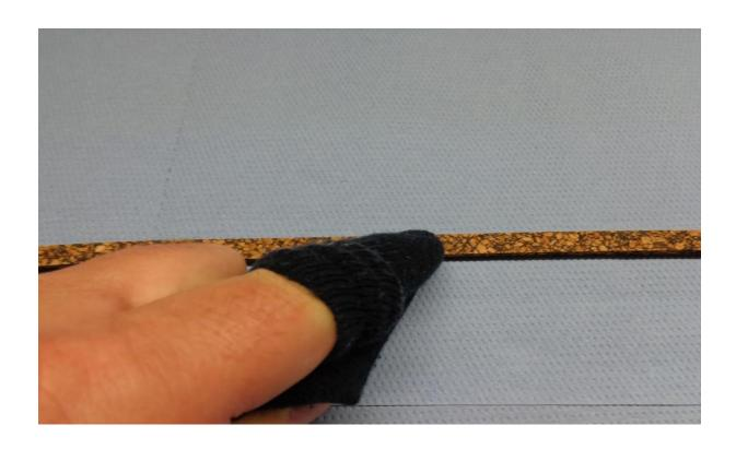
Apply the gasket on the gasket tool.
