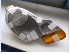
AFTER CLEANING THE BODY BY THE OLD SYLICON, PUT THE NEW SYLICON ALL AROUND THE BODY AND FIX THE EXTERNAL LENS WITH ADHESIVE PAPER TAPE. LEAVE THE LAMP IN THIS CONDITION FOR THREE DAYS.
