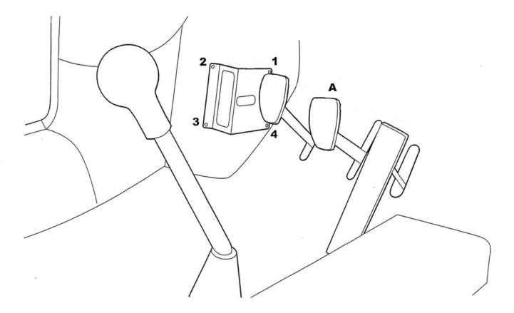
Trace an imaginary line at the top of the pedals (A) and position the top of the Dead Pedal level with this line, and the front surface flush with the clutch pedal. This position should enable you to shift your left foot between the DP and the clutch pedal with ease, and give the correct support for the left foot when you're not using it to operate the clutch. Press the DP to the left and to the front of the car at points 2 and 3, so that it sits flush on the wheel well's carpet.
