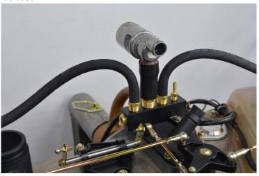
• Cut and route the 4mm silicone hose for using the resonance valve with a plenum according to the diagram below (not required for trumpets).
