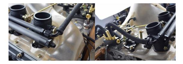
• Install the idle air control valve and 3/4" silicone hose onto the vacuum reservoir. Optional K&N filter 62-1560 may be used.
