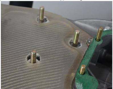
Install the four (4) studs for the oil breather cover at this time as well. The larger studs go towards the flywheel side of the engine, shown above.
